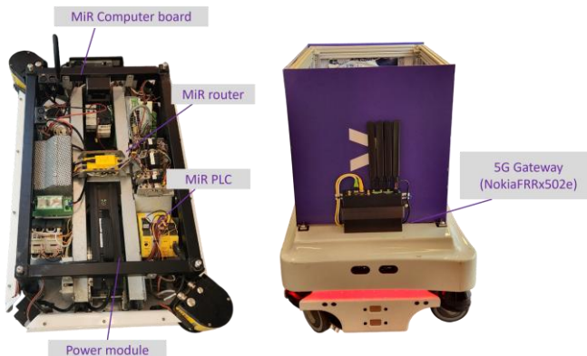
Fig. 4. 5G industrial gateway with Autonomous Mobile Robot MiR250 connected with the private 5G network.
