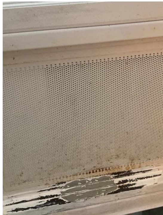
Fig. 4. Microwave oven door internally: after Repair 1.
