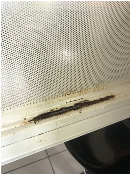
Fig. 3. Initial state of the microwave oven door.
