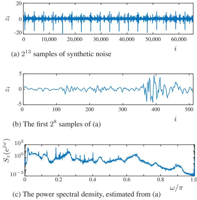
Fig. 4: Graphs of noise measured over power line.
