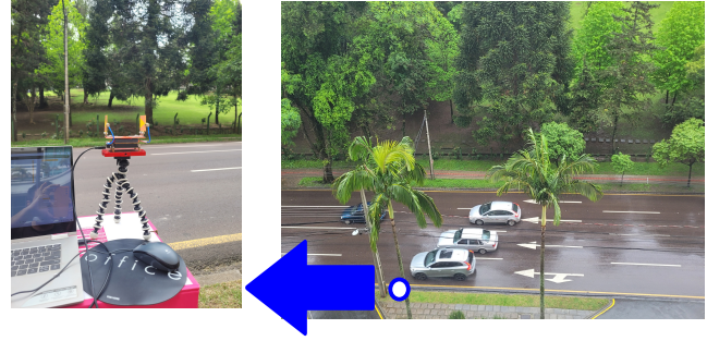
Fig. 4. Illustration of the data acquisition setup. Lanes L1 to L3 are progressively far from the radar.
