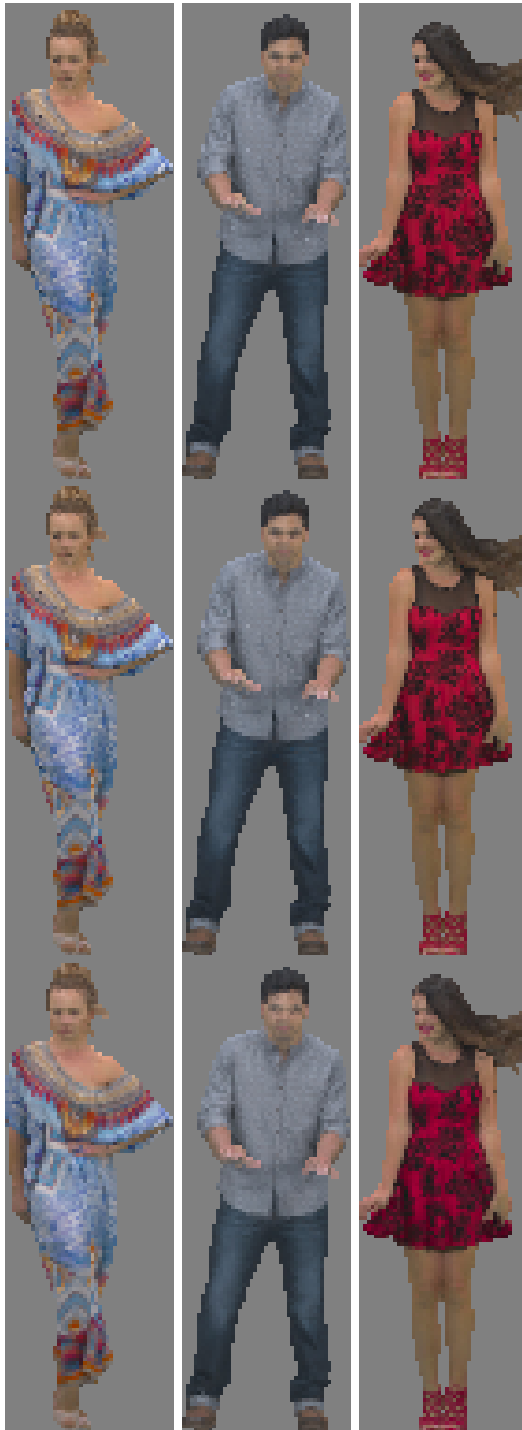
Figure 10: Subjective results for sequences Longdress_vox10_1300 , Loot_vox10_1000 and Redandblack_vox10_1450 . The first, second and third lines present results after downsampling by 8 ( K = 3 ) of: (a) the proposed method, (b) full-stream G-PCC coding and (c) no coding. For the first two methods, rate 6 of the G-PCC's CTC was applied.
