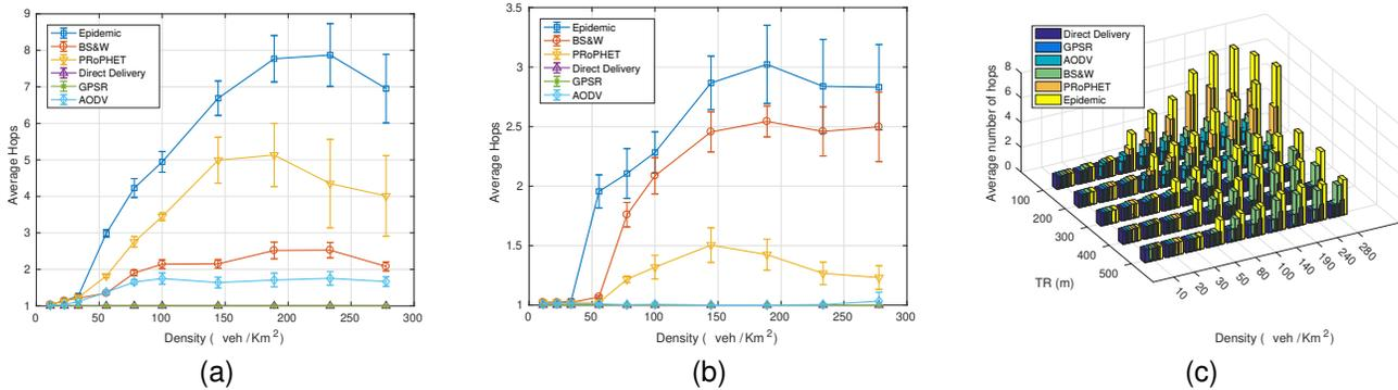
Fig. 8. Average number of hops for different transmission rates and vehicular densities. (a) TR=100 m. (b) TR=500 m. (c) TR-Density comparison.
