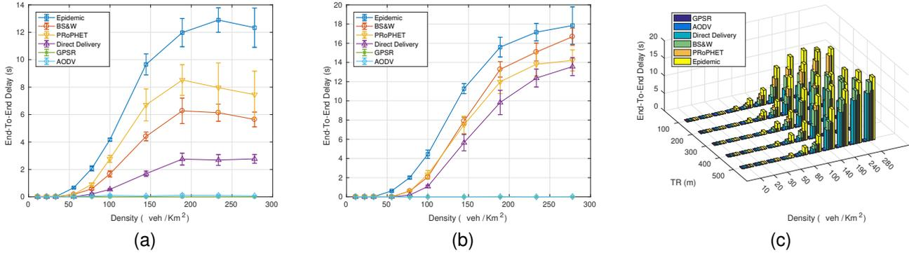
Fig. 6. Average End-To-End Delay for different transmission ranges and vehicular densities. (a) TR=100 m. (b) TR=500 m. (c) TR-Density comparison.
