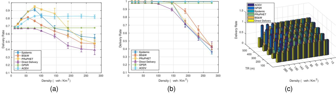
Fig. 5. Delivery Rate for different transmission ranges and vehicular densities. (a) TR=100 m. (b) TR=500 m. (c) TR-Density comparison.
