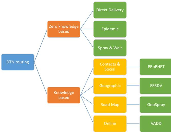
Fig. 2. Taxonomy of DTN routing protocols according to knowledge degree.
