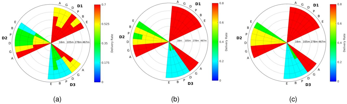
Fig. 9. Delivery Rate for different transmission ranges, distances and densities; D1=55, D2=144, and D3=233 vehicle/km<sup>2</sup>; A=AODV, G=GPSR, D=Direct Delivery, P=PRoPHET, B=Binary Spray & Wait, and E=Epidemic (a) TR=100 m. (b) TR=300 m. (c) TR=500 m.
