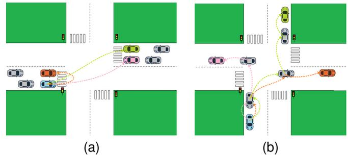
Fig. 4. Communication among four vehicles of the traffic flow. (a) Four vehicles communicate at the intersection. (b) Communication links once the traffic light opens.
