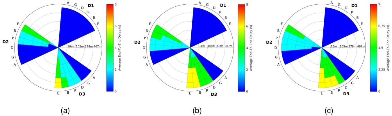
Fig. 10. Average End-To-End Delay for different transmission ranges, distances and densities; D1=55, D2=144, and D3=233 vehicle/km<sup>2</sup>; A=AODV, G=GPSR, D=Direct Delivery, P=PRoPHET, B=Binary Spray & Wait, and E=Epidemic (a) TR=100 m. (b) TR=300 m. (c) TR=500 m.
