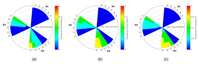
Fig. 10. Average End-To-End Delay for different transmission ranges, distances and densities; D1=55, D2=144, and D3=233 vehicle/km<sup>2</sup>; A=AODV, G=GPSR, D=Direct Delivery, P=PRoPHET, B=Binary Spray & Wait, and E=Epidemic (a) TR=100 m. (b) TR=300 m. (c) TR=500 m.
