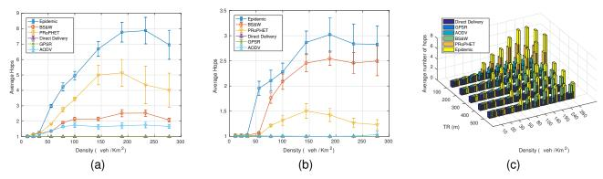
Fig. 8. Average number of hops for different transmission rates and vehicular densities. (a) TR=100 m. (b) TR=500 m. (c) TR-Density comparison.
