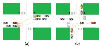
Fig. 4. Communication among four vehicles of the traffic flow. (a) Four vehicles communicate at the intersection. (b) Communication links once the traffic light opens.
