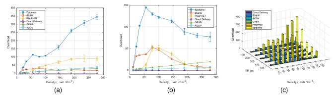
Fig. 7. Overhead for different transmission ranges and vehicular densities. (a) TR=100 m. (b) TR=500 m. (c) TR-Density comparison.
