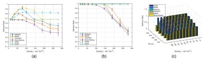
Fig. 5. Delivery Rate for different transmission ranges and vehicular densities. (a) TR=100 m. (b) TR=500 m. (c) TR-Density comparison.
