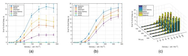
Fig. 6. Average End-To-End Delay for different transmission ranges and vehicular densities. (a) TR=100 m. (b) TR=500 m. (c) TR-Density comparison.
