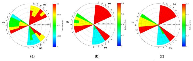
Fig. 9. Delivery Rate for different transmission ranges, distances and densities; D1=55, D2=144, and D3=233 vehicle/km<sup>2</sup>; A=AODV, G=GPSR, D=Direct Delivery, P=PRoPHET, B=Binary Spray & Wait, and E=Epidemic (a) TR=100 m. (b) TR=300 m. (c) TR=500 m.
