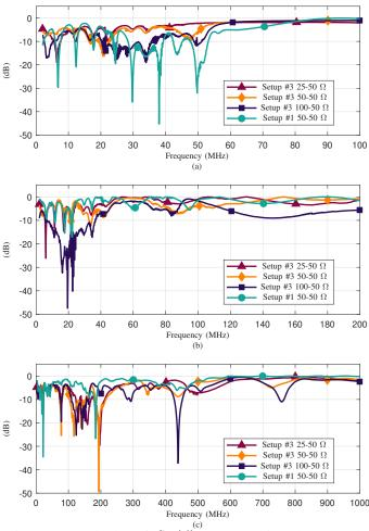
Fig. 18: Magnitudes of  $S_{11}(f)$ : A comparison between the adaptive PLC coupling circuit and the non-adaptive PLC coupling circuit of 50  $\Omega$ . (a) 2-50 MHz, (b) 2-100 MHz and (c) 2-500 MHz.
