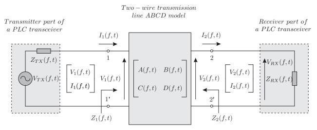
Fig. 1: Two-port ABCD time varying matrix model for dealing with the dynamic of electric power systems.
