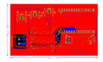
Fig. 4: The top layer of the PCB of the adaptive, broadband, capacitive, SISO and LV PLC coupling circuit.
