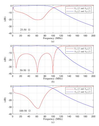
Fig. 9: Magnitude of the scattering parameter  $S_{11}(f)$ ,  $S_{22}(f)$ ,  $S_{12}(f)$  and  $S_{21}(f)$  of the analog filters designed for the adaptive PLC coupling circuit and the frequency band of 2-50 MHz. (a)  $25-50 \Omega$ , (b)  $50-50 \Omega$  and (c)  $100-50 \Omega$ .
