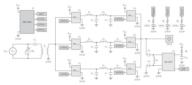
Fig. 3: The schematic of the adaptive, broadband, capacitive, SISO and LV PLC coupling circuit with J = 1 and M = 3.
