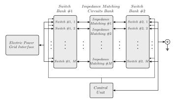
Fig. 2: The block diagram of impedance matching circuits bank for a PLC transceiver.
