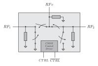
Fig. 6: The block diagram of the RF Switch PE 4239.
