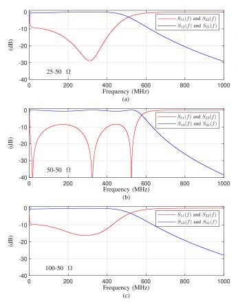
Fig. 11: Magnitude of the scattering parameter  $S_{11}(f)$ ,  $S_{22}(f)$ ,  $S_{12}(f)$  and  $S_{21}(f)$  of the analog filters designed for the adaptive PLC coupling circuit and the frequency band of 2-500 MHz. (a)  $25-50 \Omega$ , (b)  $50-50 \Omega$  and (c)  $100-50 \Omega$ .
