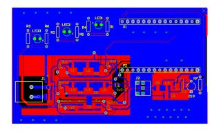
Fig. 5: The bottom layer of the PCB of the adaptive, broadband, capacitive, SISO and LV PLC coupling circuit.
