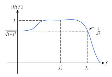
Fig. 7: Normalized frequency response of the low-pass irregular analog filter.
