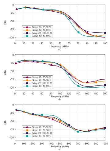
Fig. 15: Magnitudes of  $S_{21}(f)$ : A comparison between the adaptive PLC coupling circuit and the non-adaptive PLC coupling circuit of 50  $\Omega$ . (a) 2-50 MHz, (b) 2-100 MHz and (c) 2-500 MHz.
