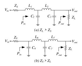
Fig. 8: The electric circuits of the designed low-pass irregular analog filters for the adaptive PLC coupling circuit.
