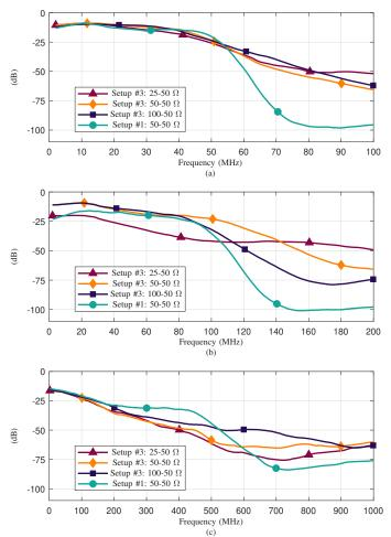
Fig. 16: Magnitudes of  $S_{21}(f)$ : A comparison between the adaptive PLC coupling circuit and non-adaptive PLC coupling circuit of 50  $\Omega$ . (a) 2 - 50 MHz, (b) 2 - 100 MHz and (c) 2 - 500 MHz.
