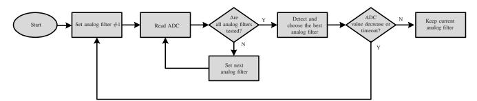
Fig. 12: Flowchart of the algorithm implemented in the Control Unit.
