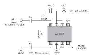
Fig. 13: Schematic of the chosen logarithmic amplifier AD 8307.
