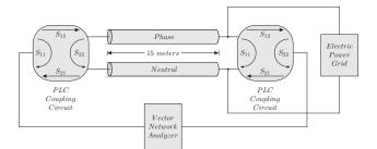
Fig. 14: The block diagram for the setup arrangement for measuring scattering parameters.
