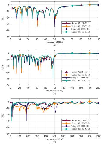
Fig. 17: Magnitudes of  $S_{11}(f)$ : A comparison between the adaptive PLC coupling circuit and the non-adaptive PLC coupling circuit of 50  $\Omega$ . (a) 2 - 50 MHz, (b) 2 - 100 MHz and (c) 2 - 500 MHz.
