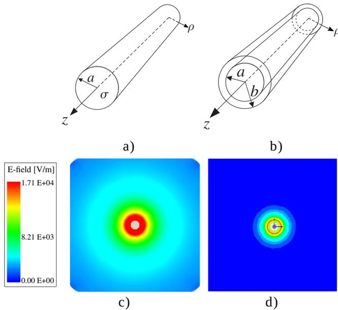
Fig. 1. Waveguides a) Sommerfeld and b) Goubau. Distribution of electric field around the guides of c) Sommerfeld and d) Goubau.
