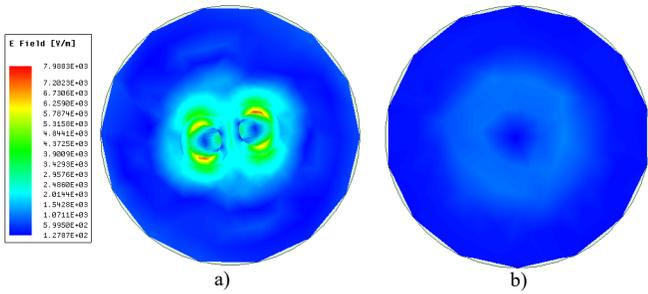
Fig. 18. Electromagnetic field in the  $P_f$  planes. a) With cable and b) Without cable.
