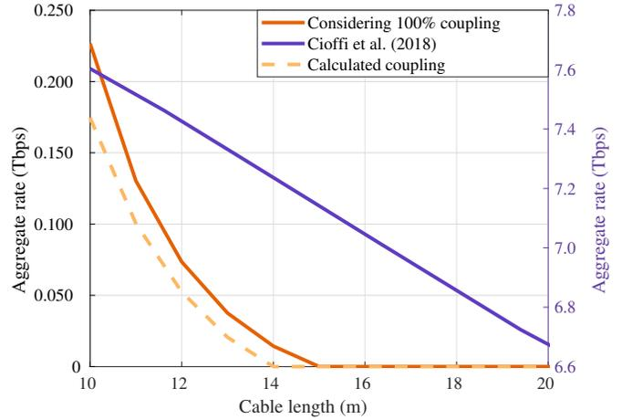
Fig. 19. Comparison of the predicted rate of this article (Calculated coupling) and that predicted in the literature, considering 100% coupling and the rate predicted by Cioffi in [4].
