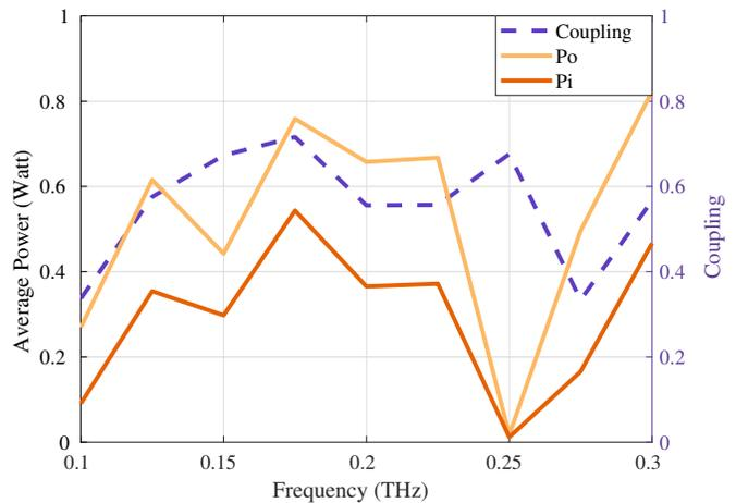
Fig. 17. Average power in the  $P_o$  and  $P_i$  planes and coupling, for antenna with new defined dimensions in 0.2 THz.
