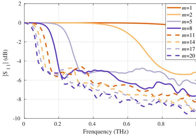
Fig. 11. Behavior of scattering parameter in function of frequency range from variation of dimension of antenna, considering the values of  $m$  equal 1, 2, 5, 8, 11, 14, 17, and 20.
