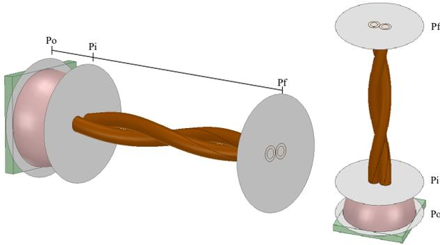
Fig. 10. Complete scenario design with measurement planes  $P_o$ ,  $P_i$  and  $P_f$ .
