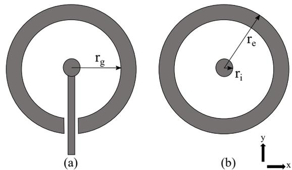
Fig. 3. Model of the photoconductive antenna proposed in [9]. (a) Real model with feeding rod. (b) Ideal model used for simulation.
