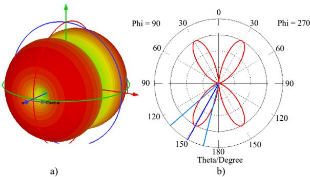
Fig. 7. (a) Far-field of the antenna simulated at 0.3 THz in free space. (b) Antenna radiation pattern with radial polarization in the y-z plane at 0.3 THz.
