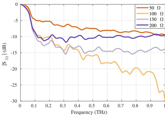
Fig. 12. Impedance variation according to the appropriate size of the antenna ( $m=20$ ) showing changes in  $|S_{11}|$  parameter level.
