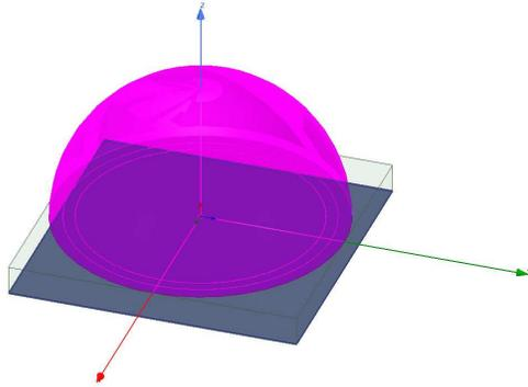
Fig. 6. Dome, substrate and antenna with PEC on the back of the substrate.
