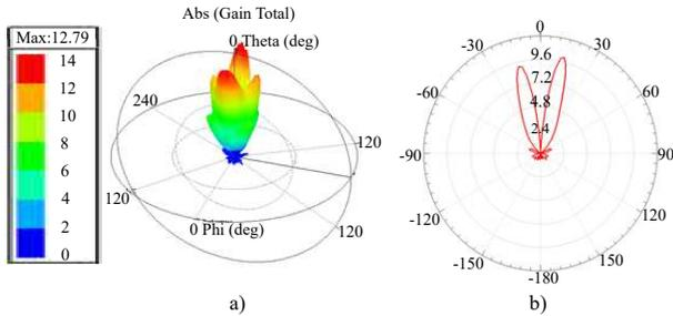
Fig. 15. a) Far-field and b) radiation diagram of the antenna with dome, substrate and PEC at the back of the substrate.
