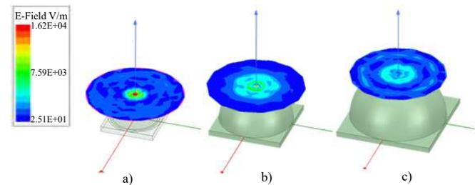
Fig. 14. Planes for measuring field concentration for different dimensions of  $n$ . a)  $n = 1.1$  b)  $n = 1.5$  c)  $n = 2$ .
