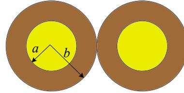
Fig. 8. Cross-section of twisted-pair.
