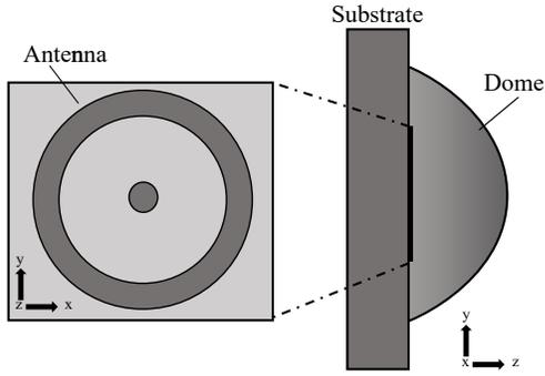
Fig. 5. Schematic representation of the antenna attached to the substrate and the coupling lens.
