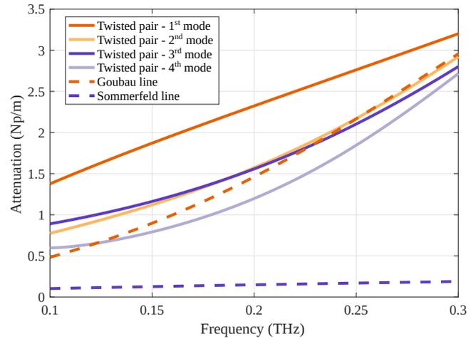
Fig. 2. Attenuation level of Sommerfeld, Goubau and twisted-pair waveguides.
