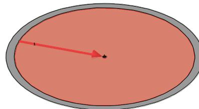
Fig. 4. Lumped port used to feed the antenna, from HFSS.
