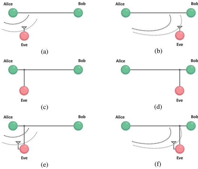
Fig. 3: Illustrations of Alice, Bob, and Eve positions. (a) SP WLC eavesdropper. (b) LP WLC eavesdropper. (c) SP PLC eavesdropper. (d) LP PLC eavesdropper. (e) SP hybrid PLC/WLC eavesdropper. (f) LP hybrid PLC/WLC eavesdropper.
