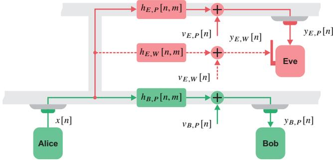
Fig. 1: Block diagram of the hybrid PLC/WLC wiretap channel model. The dashed line denotes the hybrid PLC-WLC channel while the continuous lines represent the PLC channel.
