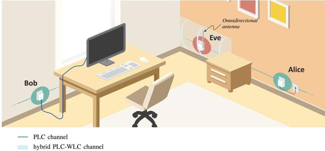
Fig. 2: Illustration of broadband data communication between two PLC devices (Alice and Bob) under the presence of a hybrid PLC/WLC eavesdropper (Eve).
