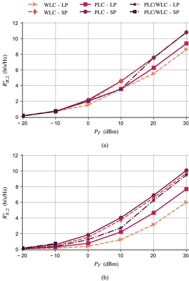
Fig. 8: Wiretap code rates in situation #2,  $R_{B,2}^*$  and  $R_{E,2}^*$ , versus total transmission power,  $P_T$ . (a)  $R_{B,2}^* \times P_T$ . (b)  $R_{E,2}^* \times P_T$ .
