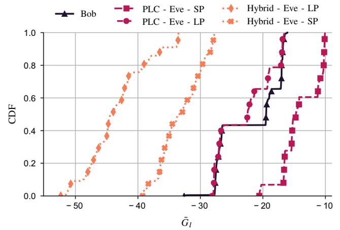
Fig. 4: Average channel gain,  $\bar{G}_l$ , of the PLC CFR estimates related to Bob and the hybrid PLC-WLC and PLC CFR estimates related to Eve in both SP and LP scenarios.
