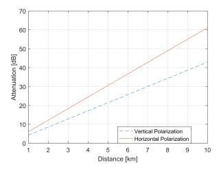
Fig. 3. Comparison between horizontal and vertical polarization.
