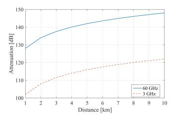
Fig. 2. Free-space loss comparison between signals operating at 3 GHz and 60 GHz.
