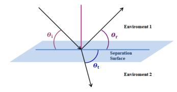
Fig. 4. Model for signal reflection and refraction.
