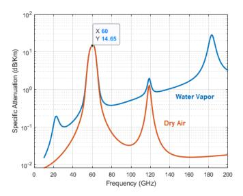
Fig. 8. Attenuation caused by dry air and water vapor as a function of the frequency. Plots obtained using Matlab 5G toolbox based on ITU-R P.676-9 [54]. Used parameter - pressure: 1013 hPa, temperature:  $15 \,^{\circ}$ C, and density: 7.5 g/m<sup>3</sup>.
