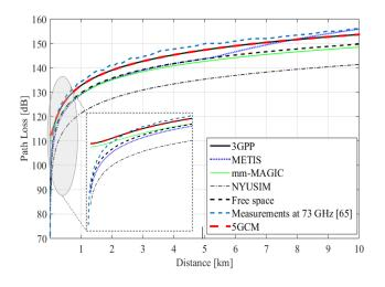
Fig. 9. Path Loss as a function of the distance between transmitter and receiver considering four different channel models in UMi scenario.
