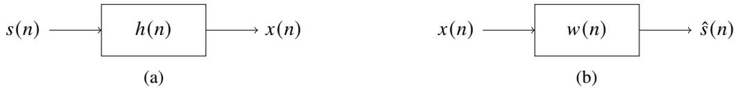
Fig. 1: (a) In the deconvolution problem, the original signal  $s(n)$  is distorted by a channel with impulse response  $h(n)$ , originating the signal  $x(n)$ . (b) Once the signal of interest has been distorted, we can adjust another filter, with impulse response  $w(n)$ , to compensate the channel distortions and produce an estimate  $\hat{s}(n)$ .
