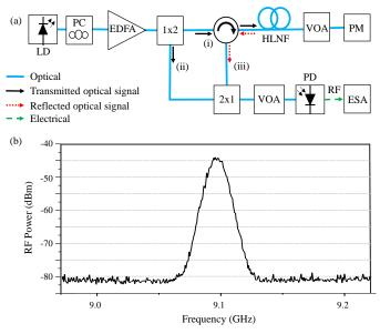
Fig. 3. Stimulated Brillouin Scattering measurement: (a) Experimental setup; (b) Measured Brillouin gain spectrum.
