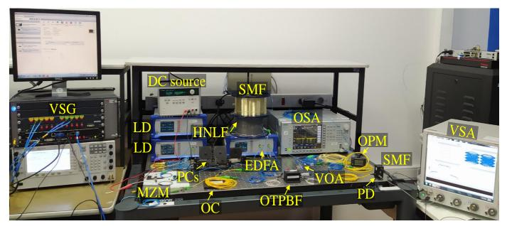
Fig. 9. Photography of the experimental setup for SBS characterization and PAA analysis.
