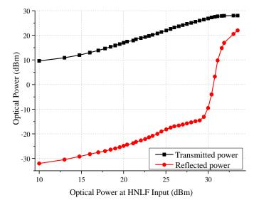
Fig. 8. Transmitted and reflected power levels as a function of the optical input power for 35 m of HNLF.
