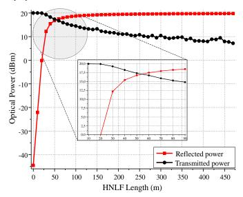
Fig. 7. Transmitted power and reflected power in the HNLF due to the SBS effect as a function of the HNLF length.
