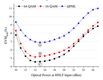
Fig. 11.  $\mathsf{EVM}_{\mathsf{RMS}}$  as a function of the optical power at the 35-meters HNLF input.
