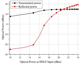
Fig. 5. Brillouin effect experimental analysis as a function of the optical input power for 470 m of HNLF.
