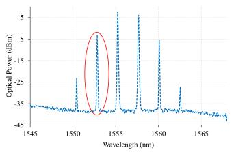
Fig. 10. Optical spectrum measured for 35 m of HNLF and the selected FWM product.
