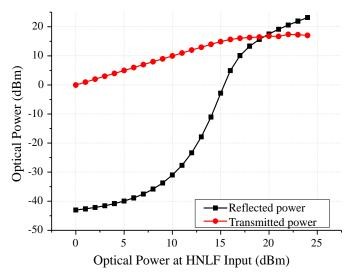
Fig. 6. Numerical analysis of the Brillouin effect as a function of the optical input power for 470 m of HNLF.
