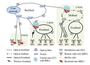
Fig. 1. The 5G X-haul vision regarding the main physical architecture.
