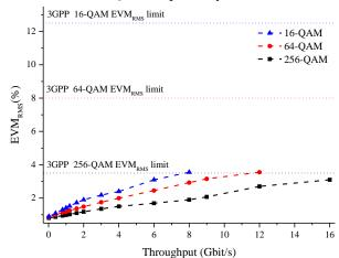
Fig. 13. Total throughput investigation as a function of  $\text{EVM}_{\text{RMS}}$  for bandwidths up to 2 GHz.
