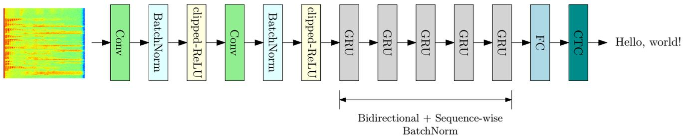
Fig. 2. DeepSpeech 2 model consisting of two convolutional (Conv) layers, each one followed by a batch normalization and clipped ReLU non-linearity, five gated-recurrent units (GRU), and one fully-connected (FC) layer, with interleaved batch-norm layers, totalling over 30 million parameters.
