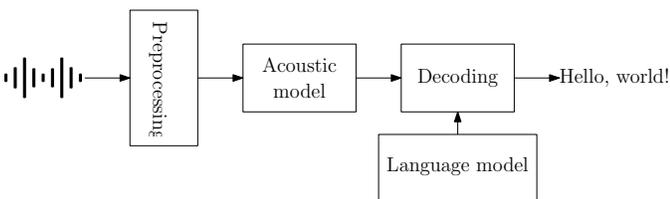
Fig. 1. The overall end-to-end automatic speech recognition system: the acoustic model is a DeepSpeech-2-based model trained using the connectionist temporal classification (CTC) loss function; the language model is an  $n$ -gram trained using the Kneser-Ney algorithm; and the decoding is the beam-search scheme adapted for the CTC algorithm.
