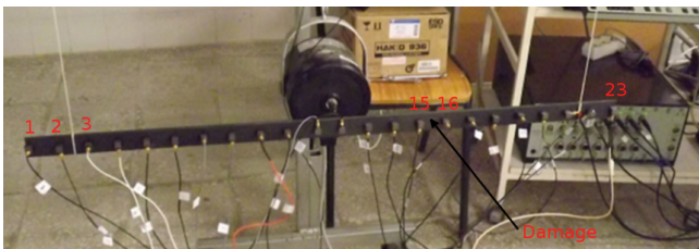
Fig. 1. Experimental setup with the identification of the accelerometers and damage location.
