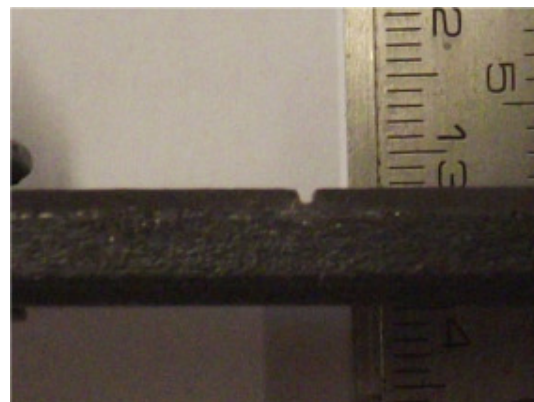
Fig. 3. Detail of the second level of damage caused by a saw cut [8].
