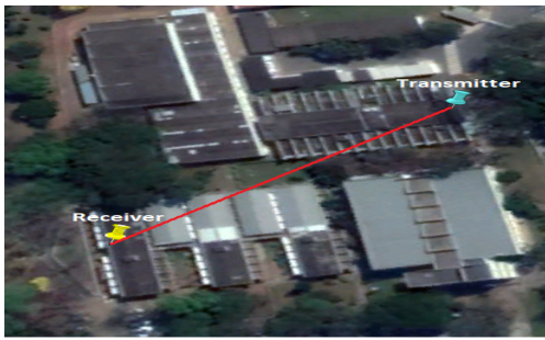
Fig. 1. Aerial view of the FSO link showing the location of the transmitter and receiver on the campus of the Faculty of Technology.
