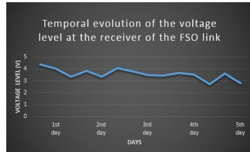
Fig. 3. Temporal behavior of the DC voltage level.
