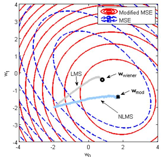
Fig. 10. Contours of the MSE and modified MSE surfaces considering the FIR channel with  $\alpha = 0.8$  and the SNR of 20 dB. The X mark refers to  $w_{\text{mod}}$ , whereas the circle represents the Wiener solution.
