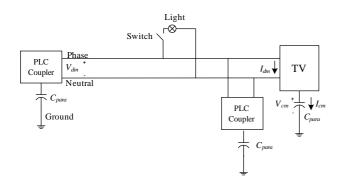
Fig. 14: High frequency equivalent circuit of a DM.
