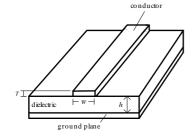
Fig. 1: A PCB microstrip transmission line.
