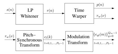
Fig. 1. Block diagram of the analysis process in ASyS.
