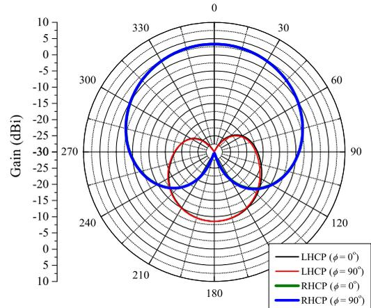
Fig. 13. Gain pattern for the antenna with four 8-cm cylindrical rods attached to each GND edge.
