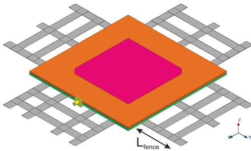
Fig. 19. Antenna structure using metallic fence.
