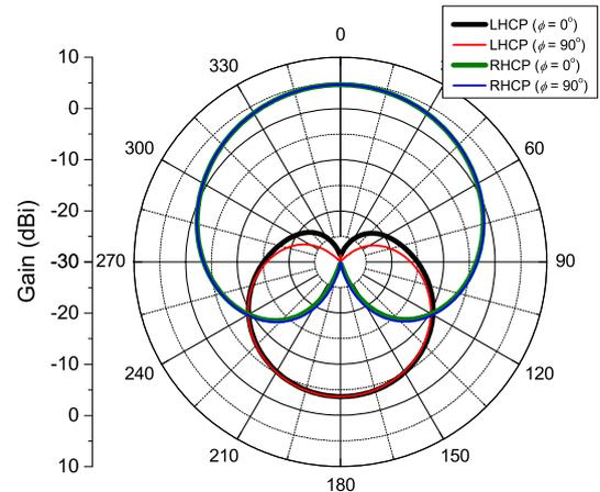
Fig. 22. Gain for the antenna with metallic fence with length of 8 cm.
