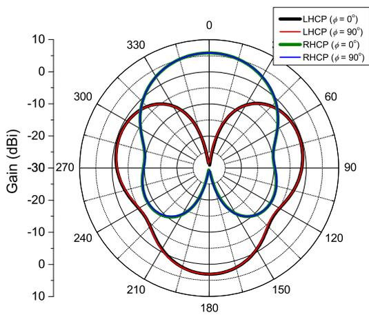
Fig. 25. Gain pattern for the antenna array with metallic fences and length of 8 cm.
