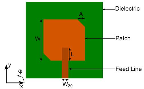
Fig. 3. Schematic top view of the designed antenna.
