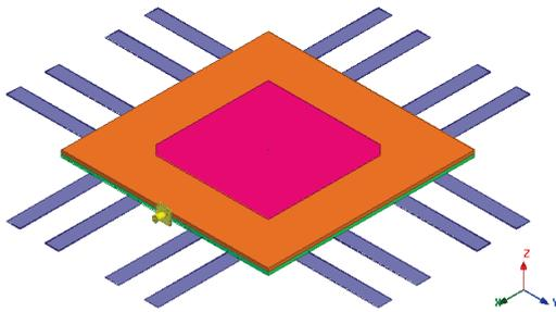
Fig. 14. Designed antenna with metallic strips.
