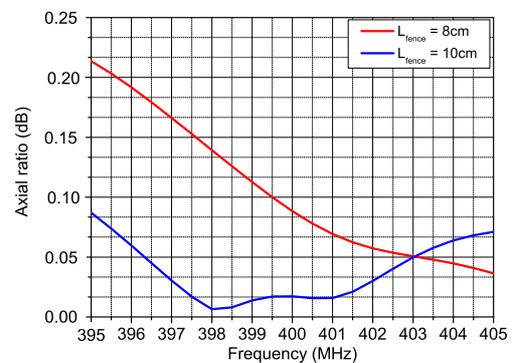
Fig. 28. Axial ratio as a function of the frequency for the antenna array with metallic fence model.
