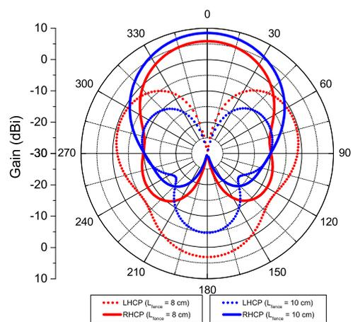
Fig. 29. Gain for the antenna array with metallic fences considering  $L_{fence} = 8$  cm and  $L_{fence} = 10$  cm.
