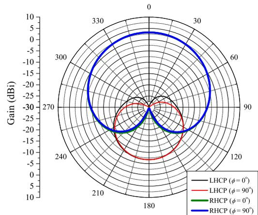
Fig. 17. Gain for the antenna with two metallic strips and length of 8 cm.
