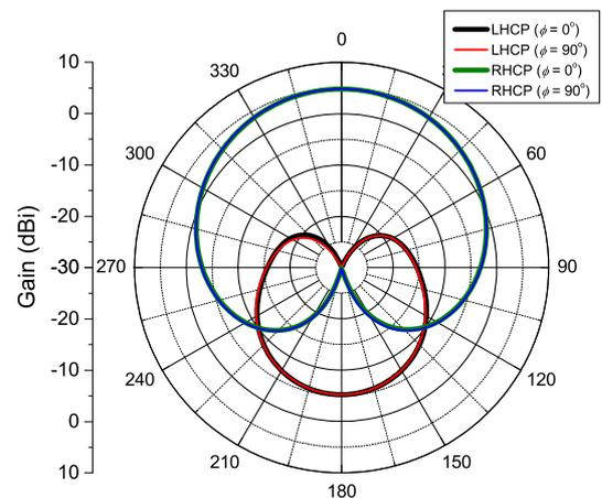
Fig. 23. Gain for the antenna with metallic fence with length of 10 cm.
