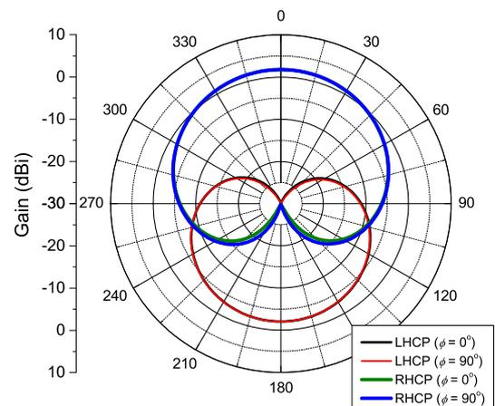
Fig. 5. Gain pattern for the standard antenna.
