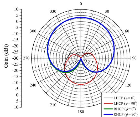
Fig. 18. Gain for the antenna with four metallic strips and length of 8 cm.
