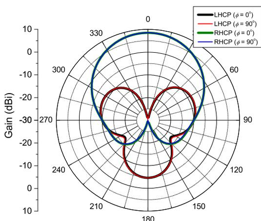
Fig. 26. Gain for the antenna array with metallic fences with length of 10 cm.
