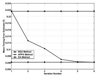
(a) Mean Timing Estimate versus Iteration Numbers for NDA, APPA and DA Timing Estimation Methods with  $E_b/N_0 = 1.5$  dB and Timing Offset = 0.2T, BPSK Modulation.
