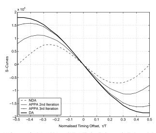
(a) S-curves for DA, APPA, and NDA Timing Estimators in Turbo-coded BPSK System with  $E_b/N_0 = 2$  dB, and Timing Offset=0.0.
