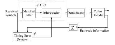
Fig. 3. Block Diagram of a Receiver Using the APPA Timing Recovery in a Turbo Coding System.
