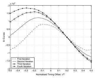
(b) S-curves for APPA Timing Estimator in Turbo-coded BPSK System with 4 Different Iterations,  $E_b/N_0 = 2$  dB, and Timing Offset=0.2T.
