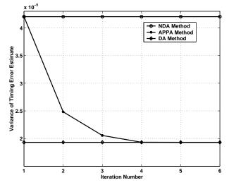
(b) Variance of the Timing Estimation versus Iteration Numbers for NDA, APPA and DA Timing Estimation Methods with  $E_b/N_0 = 2 \text{ dB}$  and Timing Offset = 0.2T, BPSK Modulation.
