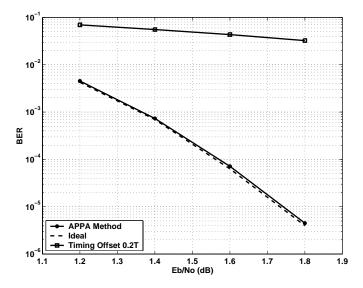
Fig. 7. BER Performance versus  $E_b/N_0$  using APPA Timing Estimation Method for Turbo-coded BPSK System after Six Iterations with Timing Offset 0.2T.
