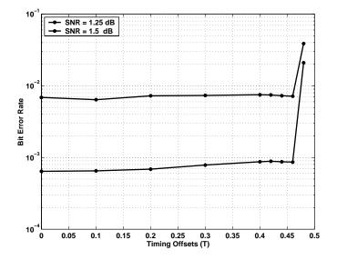
Fig. 6. BER Performance versus Timing Offsets using APPA Timing Estimation Method for Turbo-coded BPSK System after Four Iterations for  $E_b/N_0$ =1.25 dB and 1.5 dB.
