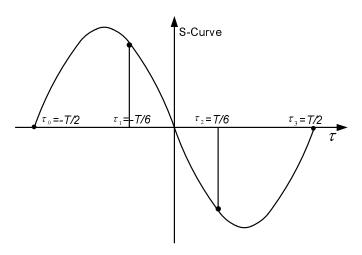
Fig. 2. Four Samples at  $\{-T/2, -T/6, T/6, T/2\}$  on the S-curve Used by the Linear Interpolation Algorithm to Determine the ML Timing Estimate
