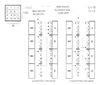
Figura 15. Collision-free interleaver generation from matrix M.
