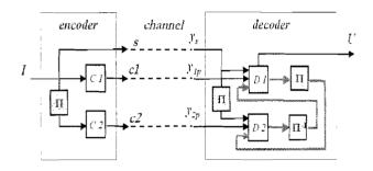
Figure 1. General turbo coding scheme.
