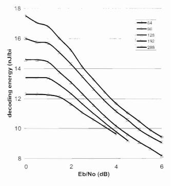
Figure 23. Measured core energy consumption
