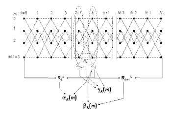
Figure 2. Metrics of the MAP decoding algorithm.
