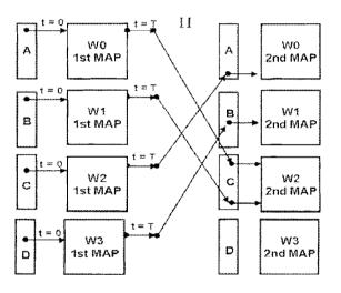
**Figura 14.** Representation of a collision when accessing storing elements in the MAP parallel decoder architecture.
