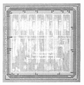
Figure 20. Eletromiography of the processed core showing the turbo codec main building blocks.
