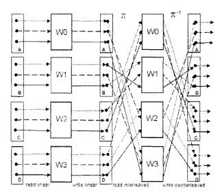
Figure 19. Optimized parallel turbo decoding schedule.
