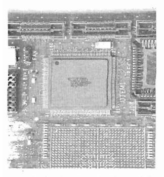
**Figure 22** The turbo codec ASIC (nick-named 'T $(\hat{a}$  MPO' Turbo ( $\hat{a}$  Minimum Power) inserted on the test board.
