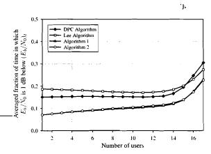
(a) Actuation period of the power control 2 ms and Doppler spread 18.5 Hz.
