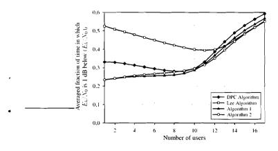
(a) Actuation period of the power control 2 ms and Doppler spread 55.5 Hz.
