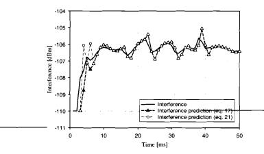
**Figure 2.** Comparison between actual and predicted interference using the proposed prediction methods, for the Doppler spread 18.5 Hz.
