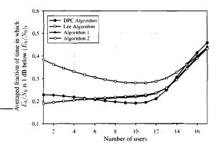
(b) Actuation period of the power control 4 ms and Doppler spread 18.5 Hz.
