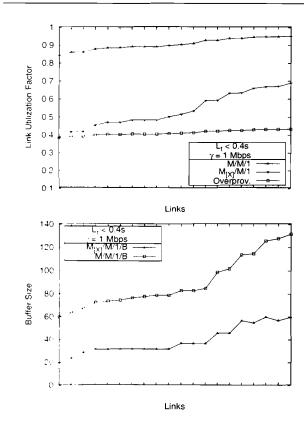
Figure 5. Link utilization factor and Buffer size for the 10node network (classical and new approach)
