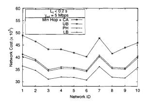
Figure 6. Network cost for 40-node networks with random topologies (considering: Lagrangean relaxation (LB), primal heuristic with logarithmic barrier CA solution (PH), primal heuristic with approximate CA solution (UB), CA with minimum-hop routing (MinHop+CA)
