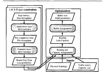
Figure 1. Schematic Flow Diagram of the Network Design Methodology
