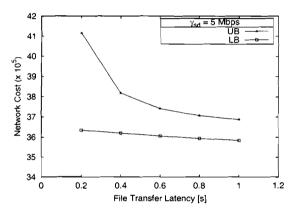
Figure 7. LB and UB network costs as a function of latency constraints (40-node, 160-link network)
