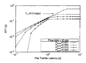
Figure 2. Maximum admissible RTT which satisfies the most stringent constraint (latency or throughput) for different values of  $P_{loss}$  (considering 20-packet flows)
