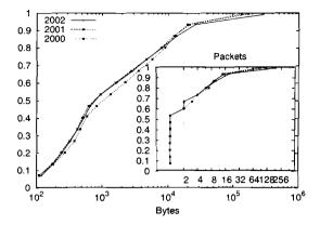
**Figure 3**. TCP connection length cumulative distribution derived from one-week long measurements in three different time periods
