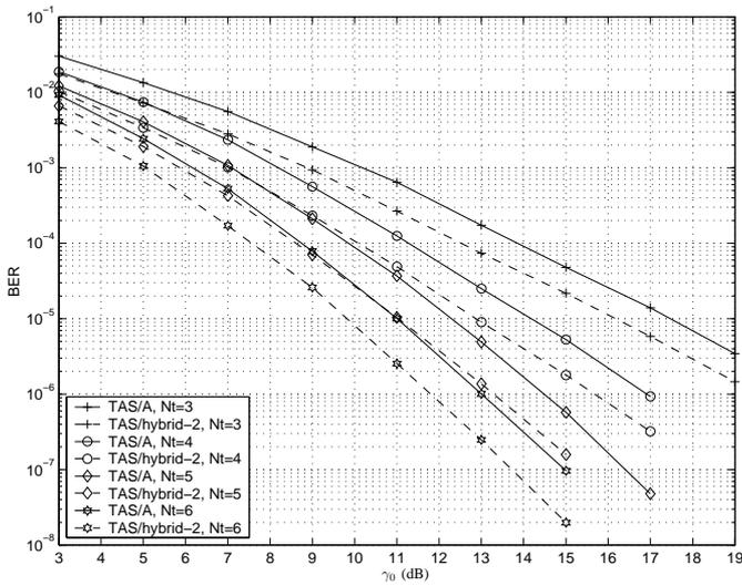
Fig. 4. BER of TAS/hybrid-2 ( $n_t = 1$  or 3) and TAS/A ( $n_t = 2$ ) for BPSK,  $N_t = 3, \dots, 6$ , and  $N_r = 1$ . Full (i.e., order  $N_t$ ) diversity is achieved as if all the transmit antennas were used.
