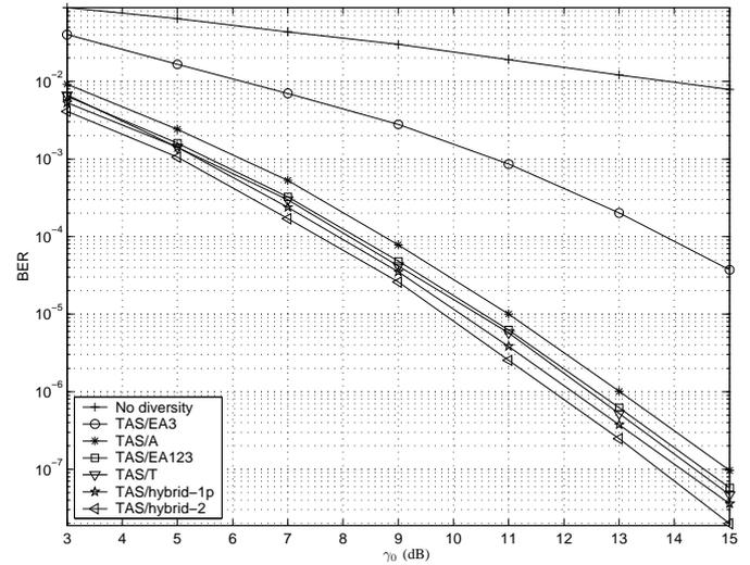
Fig. 3. BER of TAS/EA3, TAS/A, TAS/EA123, TAS/T, TAS/hybrid-1p, and TAS/hybrid-2, for BPSK,  $N_t = 6$ , and  $N_r = 1$ .
