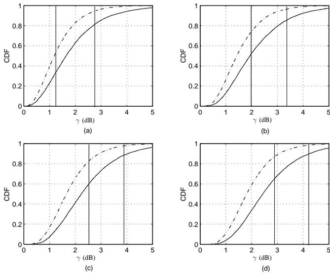
Fig. 1. CDF of  $\gamma_{TAS/hybrid-2}$  (solid lines) and  $\gamma_{TAS/A}$  (dashed lines) for (a)  $N_t = 3$ , (b)  $N_t = 4$ , (c)  $N_t = 5$ , and (d)  $N_t = 6$  transmit antennas, and  $\gamma_0 = 1$  (0 dB). Vertical lines indicate average SNRs.  $N_r = 1$ .
