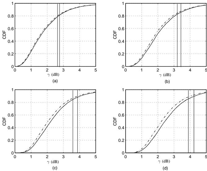
Fig. 2. CDF of  $\gamma_{TAS/hybrid-2}$  (solid lines) and  $\gamma_{TAS/T}$  (dashed lines) for (a)  $N_t = 3$ , (b)  $N_t = 4$ , (c)  $N_t = 5$ , and (d)  $N_t = 6$  transmit antennas, and  $\gamma_0 = 1$  (0 dB). Vertical lines indicate average SNRs.  $N_r = 1$ .
