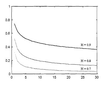
Figure 3. Autocorrelation function r(k)
