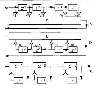
Figure 2. ARIMA(p,d,q)filter scheme.
