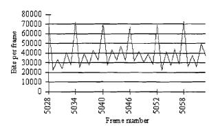
**Figure 1.** Classic pattern of the bits per frame generated by a VBR MPEG coder with (Q=6, M=2, N=6) set parameters.
