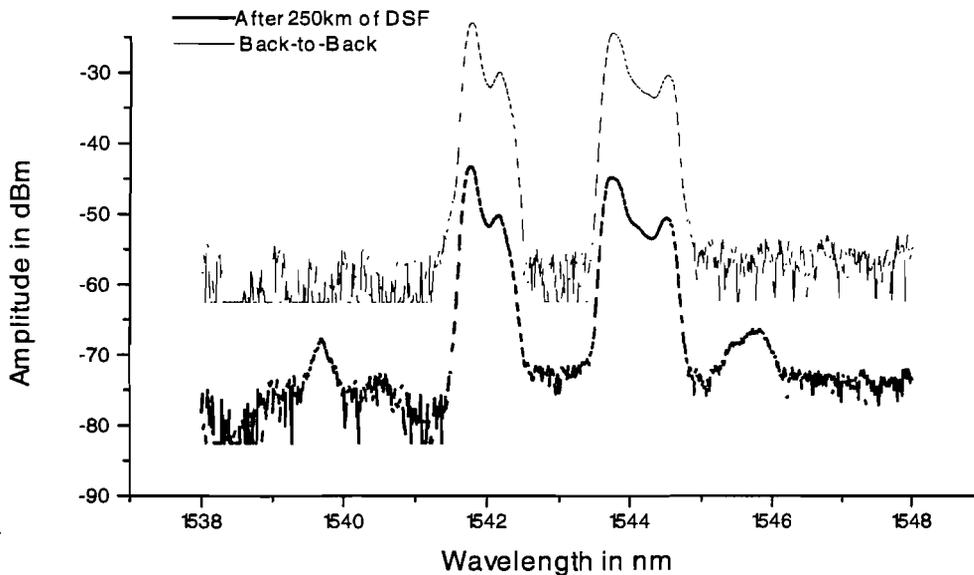
**Fig 3 Optical spectrum after 250km of propagation through DSF. The output of the booster amplifier is set to +24dBm**
