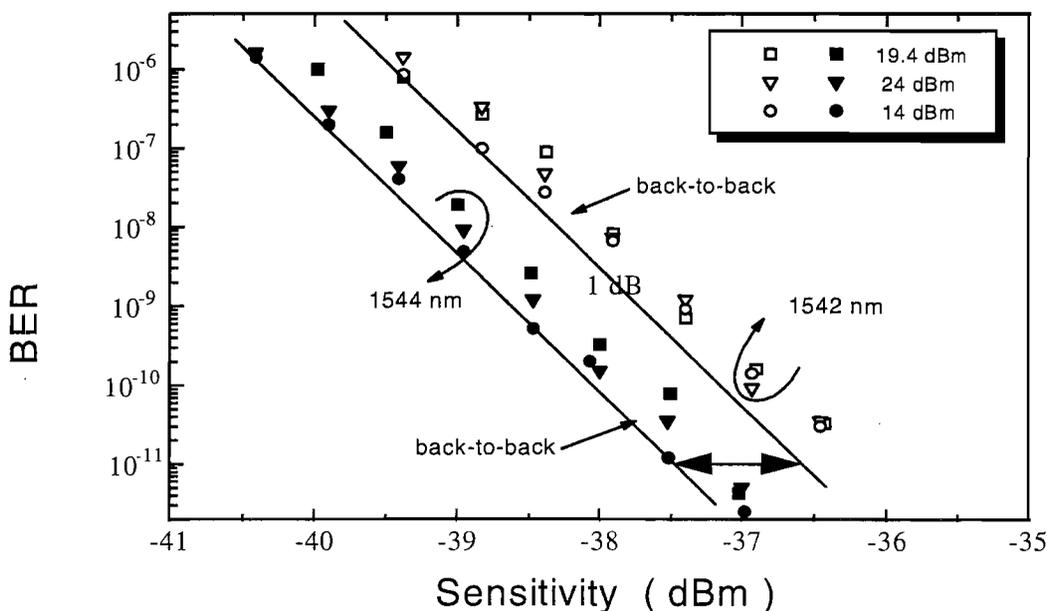
Fig. 2 BER versus receiver sensitivity for both channels at three different transmitter power levels
