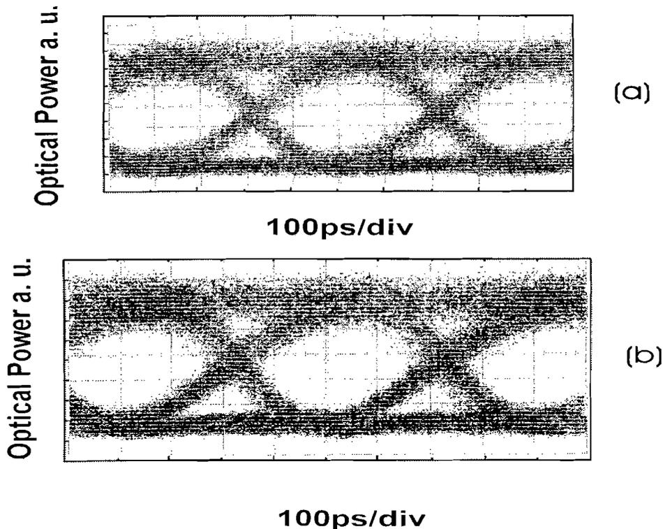
Fig 4 Eye diagram of both channels after 250km transmitted through DSF. (a) 1542nm, (b) 1544nm
