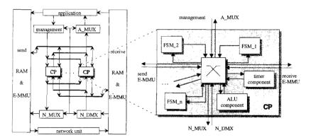
Figure 2 - Overview of the VLSI implementation architecture
