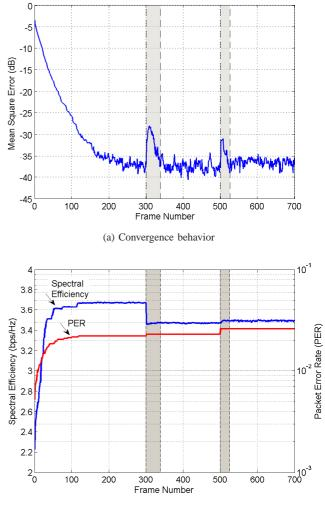
(b) Spectral efficiency and packet error rateFig. 7: Convergence behavior, spectral efficiency and packet error rate of the
