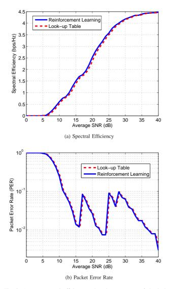
Fig. 2: Average spectral efficiency and packet error rate of the look-up table and the reinforcement learning technique under the suburban macrocell scenario.
