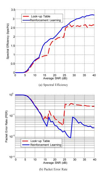
Fig. 8: Average spectral efficiency and packet error rate of the look-up table and the reinforcement learning technique under the suburban macrocell scenario considering the presence of RF imperfections on the receiver side.
