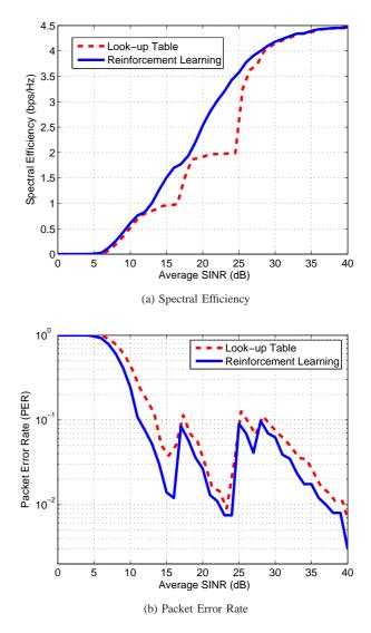
Fig. 5: Average spectral efficiency and packet error rate of the look-up table and the reinforcement learning technique under the suburban macrocell scenario and colored interference. The interference power is three times higher than the white noise variance.
