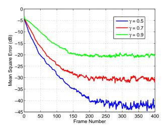
Fig. 3: Influence of the discount factor  $\gamma$  on the convergence of the RL algorithm for  $\epsilon_i=0.95$  and  $\epsilon_f=0.05.$
