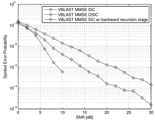
Fig. 3. Average SEP performance comparison of SIC, OSIC and SIC with backward recursion detectors.
