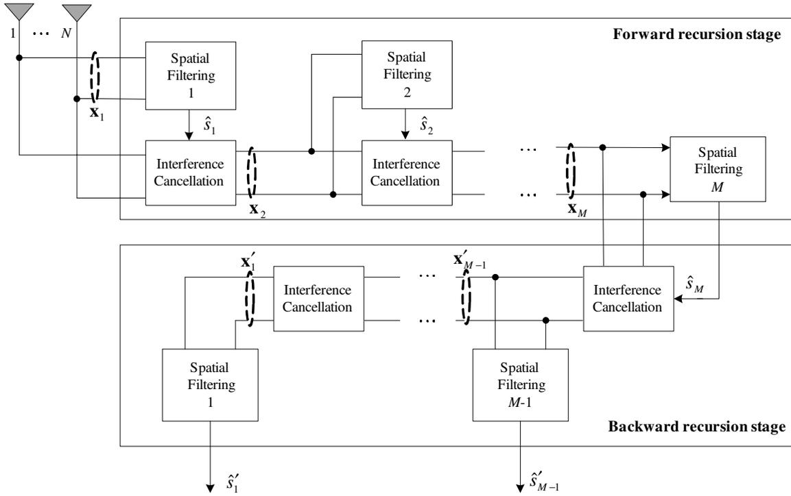
Fig. 1. Structure of SIC receiver with backward recursion processing.
