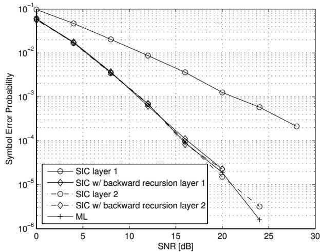
Fig. 2. SEP performance per layer of SIC receiver with and without backward recursion and ML detectors.
