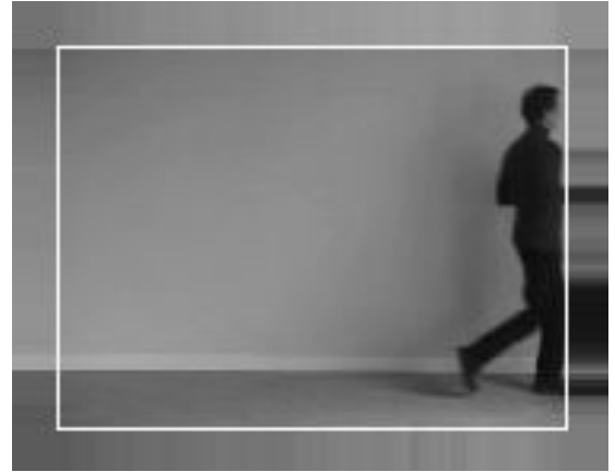
Fig. 6. Treatment for out-of-bounds block coordinates. The white rectangle highlights the original frame. Intensity values for pixels outside of this rectangle are the same as those in the border.
